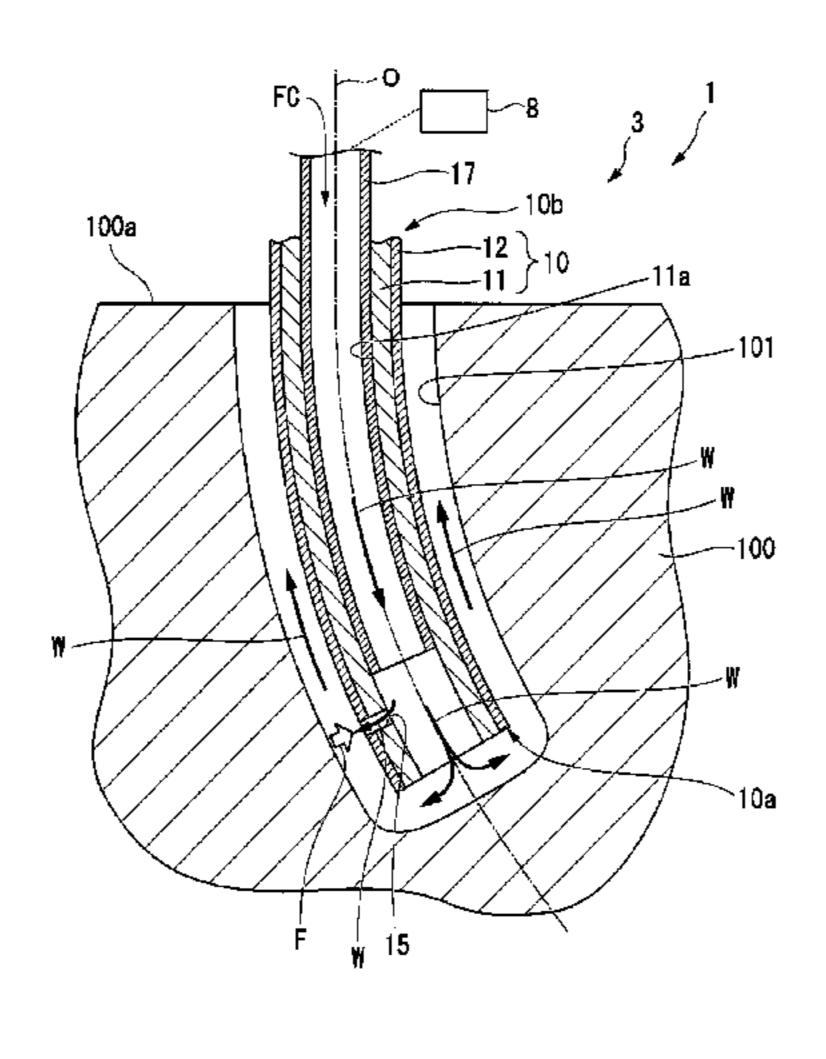
tool body in a radial direction and guiding the electrolytic solution flowing through the flow channel outward in the radial direction, and the electrochemical machining tool further comprises a tube-shaped member selectively opening and closing the fluid outflow hole.
