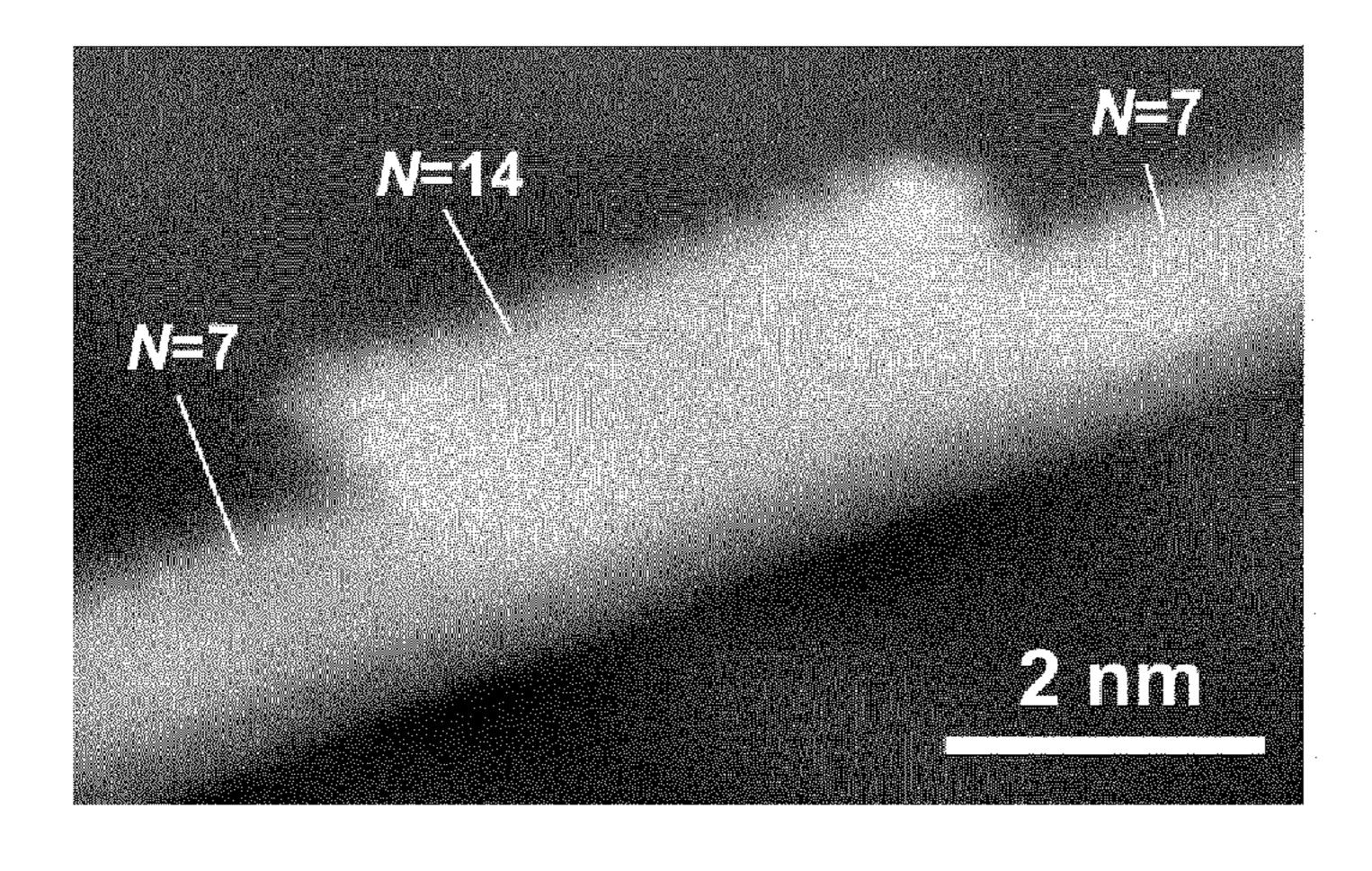
segment width of at least one of said graphene segments is 4 nm or less and to a method for preparing it by polymerizing at least one polycyclic aromatic monomer compound and/or at least one oligo phenylene aromatic hydrocarbon monomer compound to form at least one polymer and by at least partially cyclodehydrogenating the one or more polymer.
