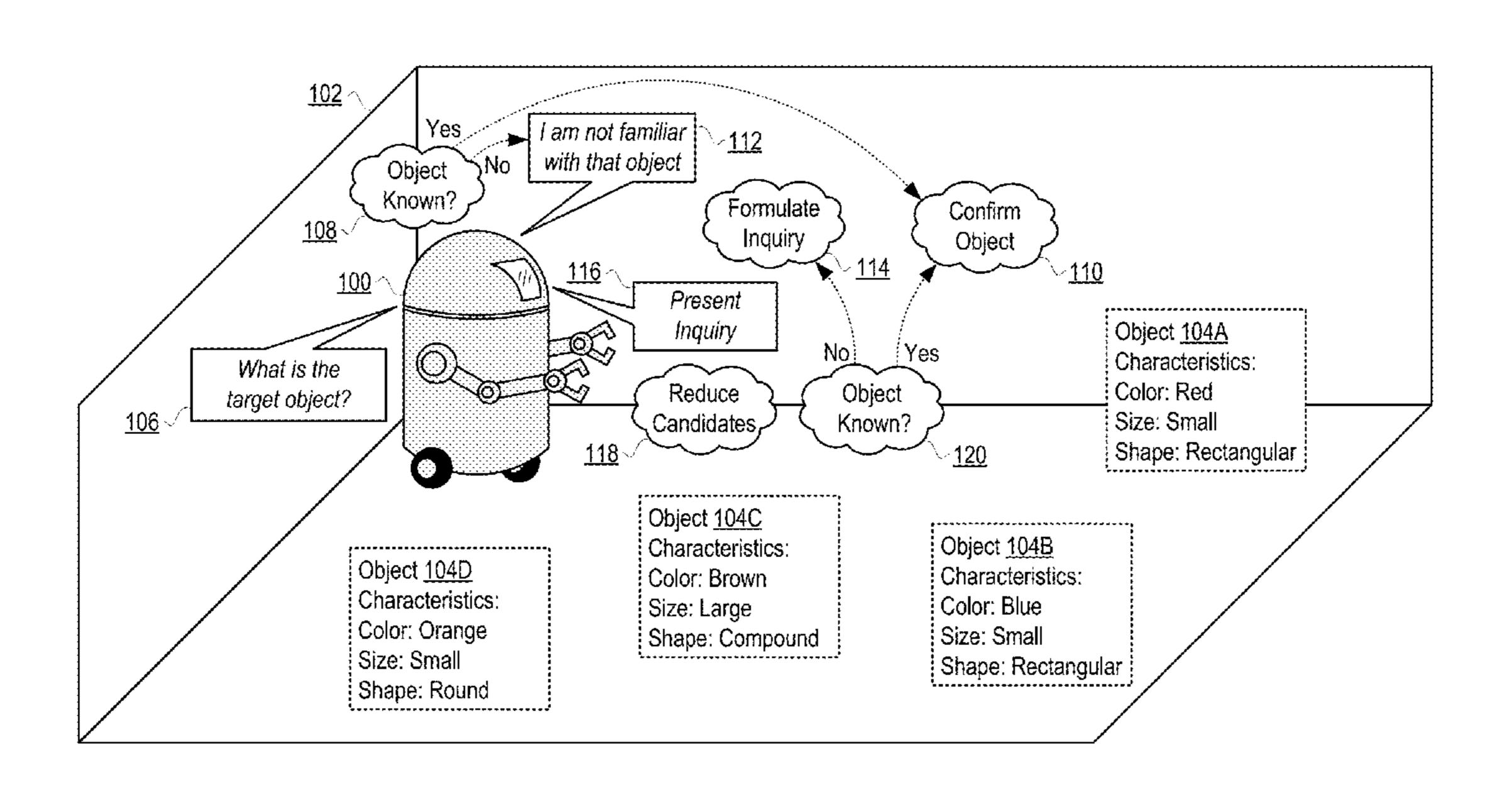
target objects, and may select a characteristic that most substantially reduces a number of potential target objects. After the characteristic is determined, the device may formulate an inquiry to the user utilizing the characteristic. Characteristics may be selected until the device determines the target object and confirms it to the user.
