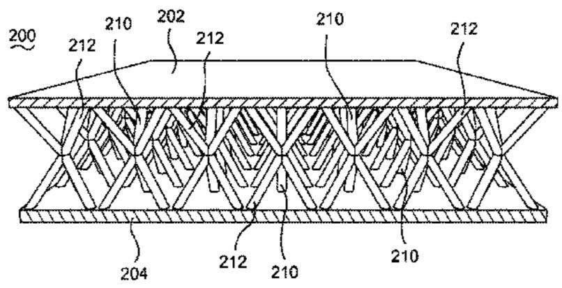
the mold core, filling the mold core with a liquid alloy to cast and directionally solidify the truss structure.
