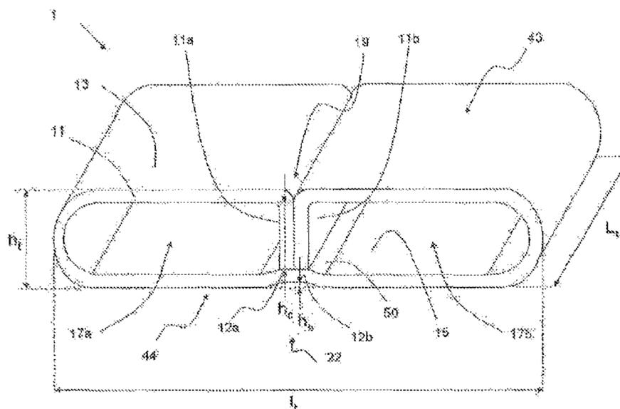
the metal strip (11) in order to form said heat exchanger tube (1), such that the projection extends into the tube (1). The invention also relates to such a tube (1) and to a heat exchanger (3) comprising a bundle of said tubes (1).
