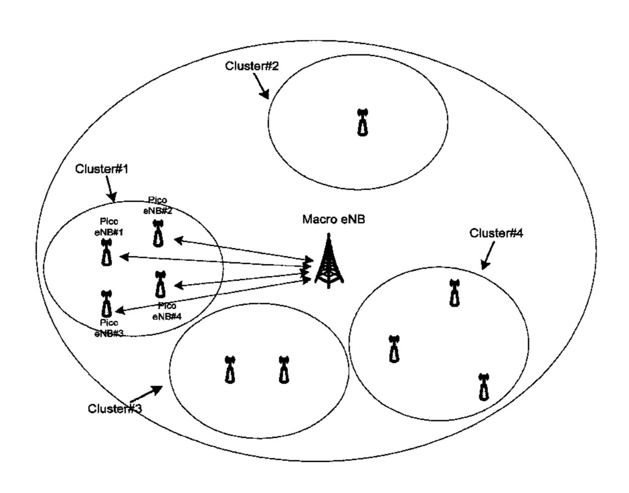
cell of the cell cluster out of a set of predefined uplinkdownlink configurations with flexible subframe patterns for flexible time division duplex communication on the basis of the specified desired uplink-downlink configuration for the subject cell and the obtained at least one desired uplinkdownlink configuration for the at least one neighboring cell.
