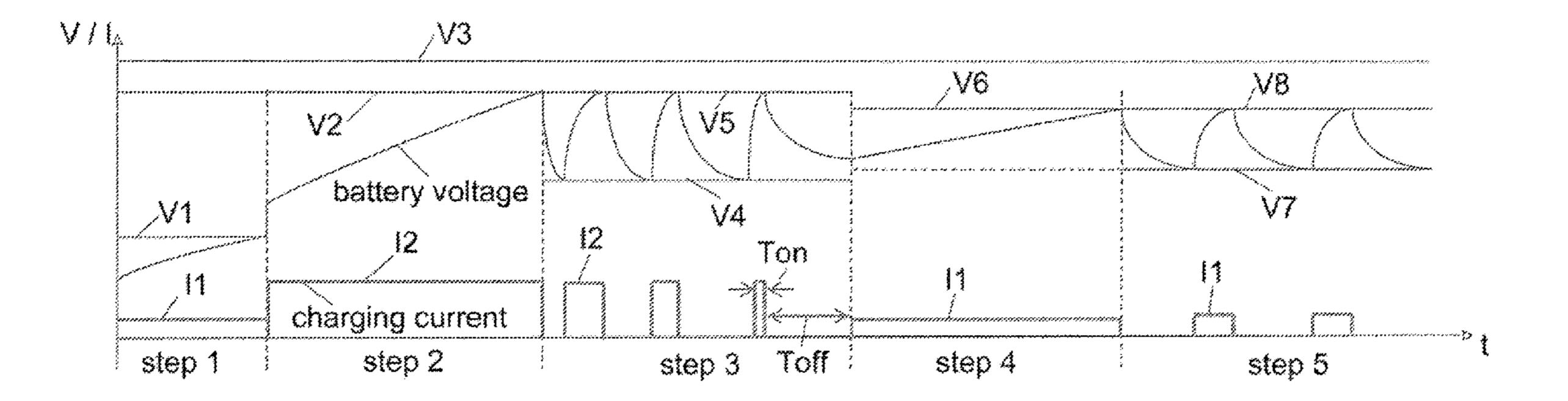
a fifth voltage threshold (V5), and wherein said third charging step providing said repeated switching on and off the third constant charging current (I3) thereby producing current pulses ends if the length of a current pause (Toff) following said current pulse (Ton) equals or exceeds the length of p·(k-1)-times the preceding current pulse (Ton) with k being the ratio of constant charging current I3 and the constant charging current I1 and p being a defined factor.
