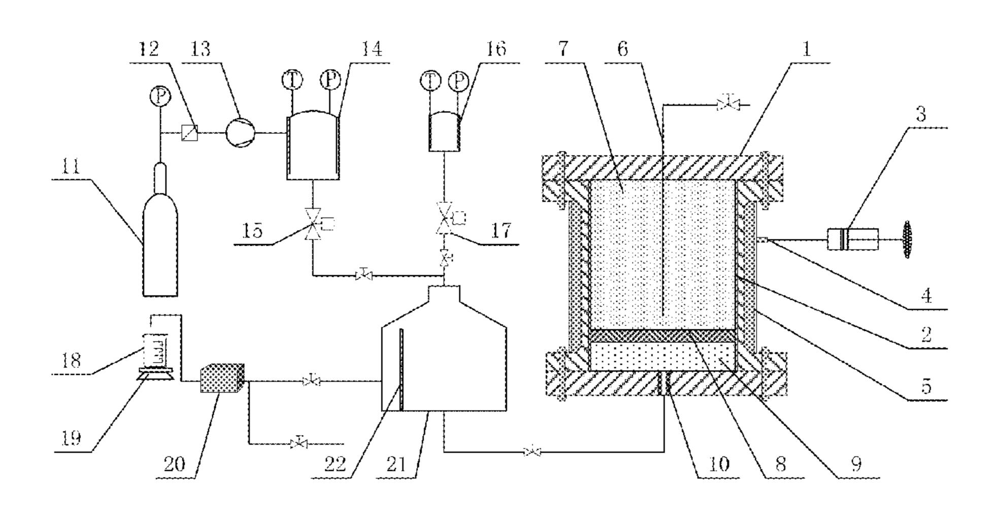
the high pressure reaction kettle is connected with liquid injection, gas injection, gas production and water production equipment. An aquifer interface at the bottom of the high pressure reaction kettle is connected to the aquifer maintaining unit through a pipeline. The simulation device simulates the geological environment of a hydrate reservoir, allowing comprehensive evaluation of hydrate exploitation under different formation permeability and different formation pressure gradients.
