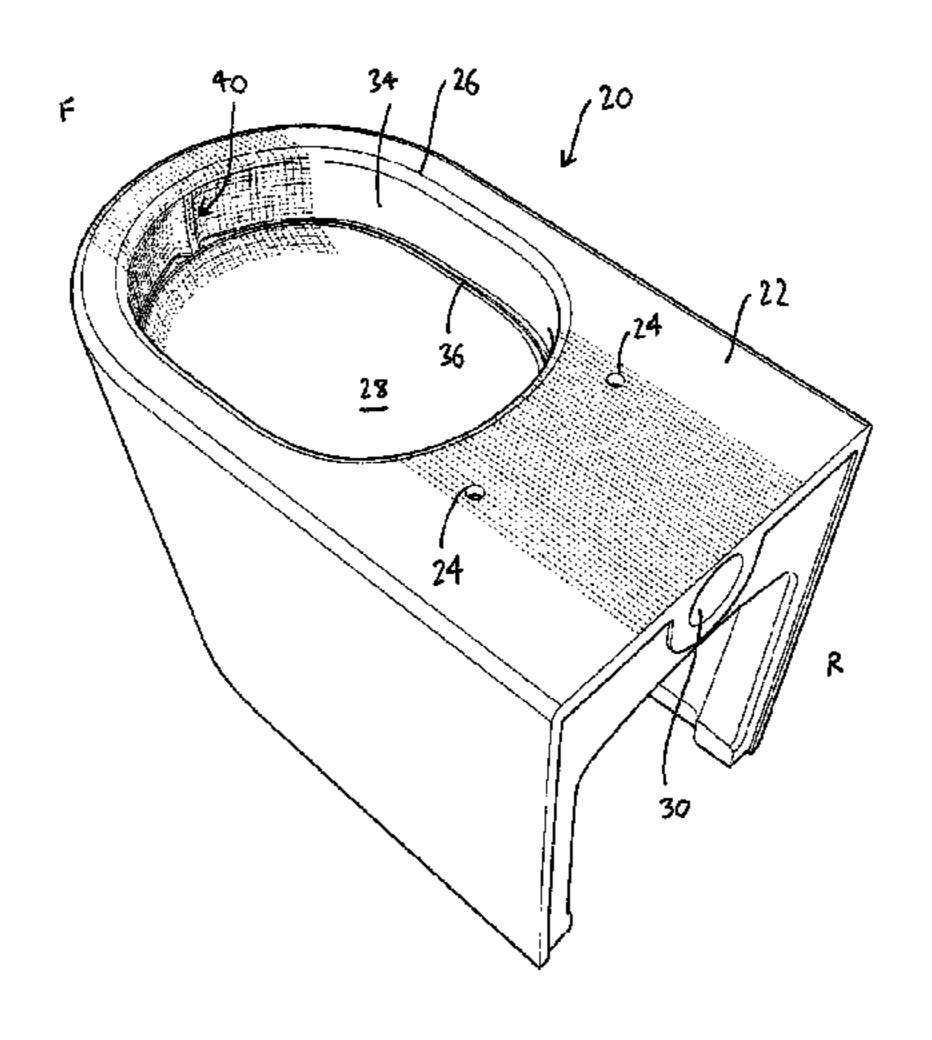
sidewall (34) and is positioned substantially symmetrically in relation to a forward to rearward centerline (42) of the toilet pan (28).
