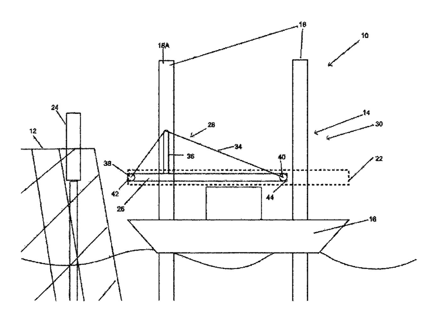
The/each compression post supports the cable between the cable first end and the cable second end and is adapted to maintain a substantially constant tension in one of said cables as the platform moves from the stowed position to the extended position.
