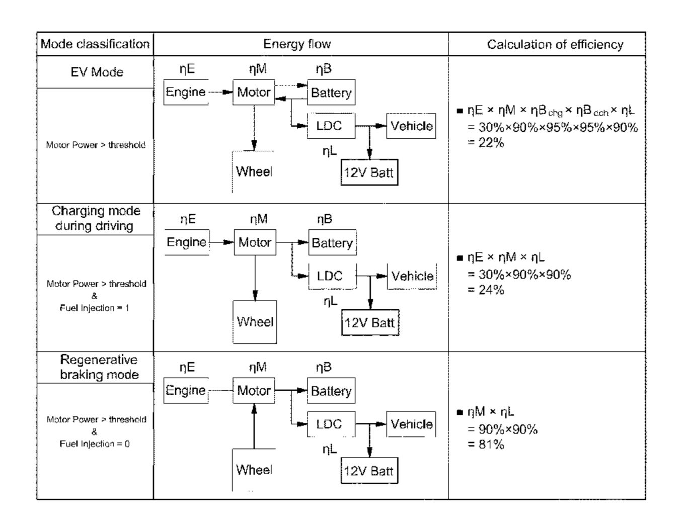
mode is switched from the regenerative braking mode to an electric vehicle (EV) mode, and to variably adjust an LDC target voltage in the EV mode.
