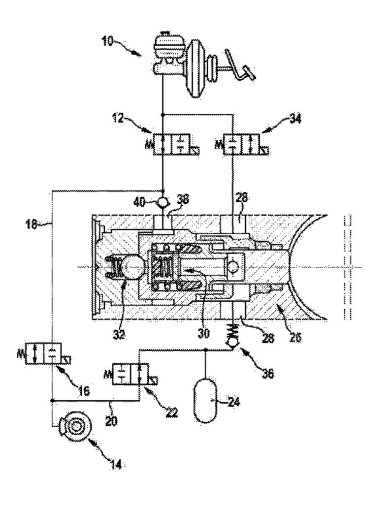
outlet valve which prevents an exerting of the pressure generator on the pressure side with the pressure of the main brake cylinder.
