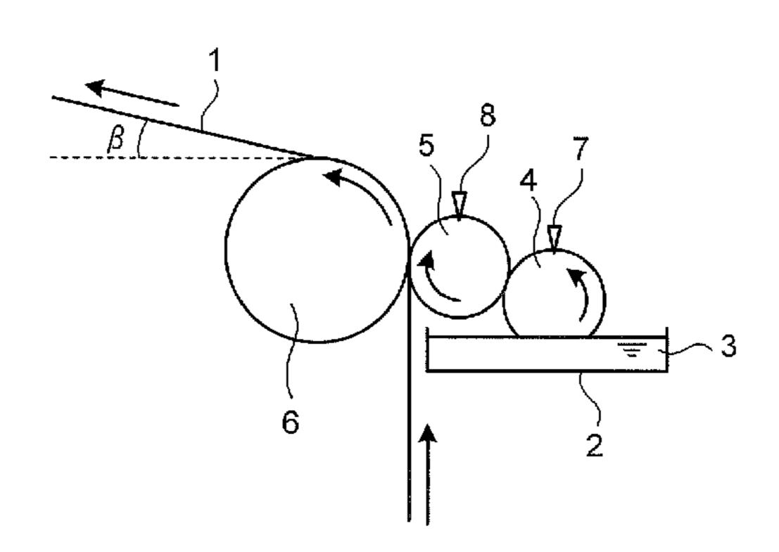
tion liquid to a steel strip; and a second scratch off member configured to scratch off the application liquid from the roll surface of the second roll.
