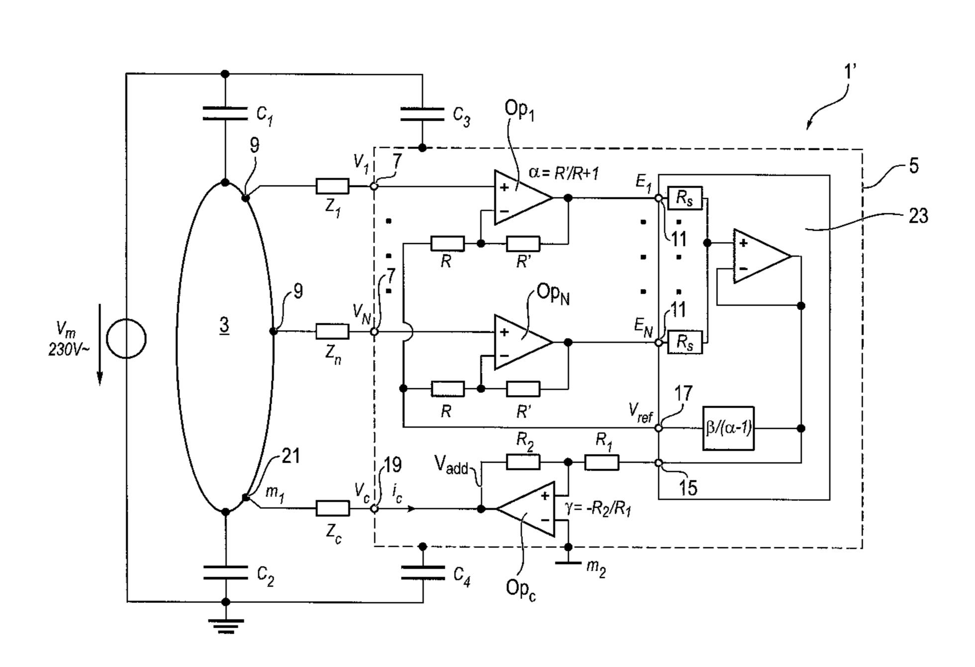
each measuring amplifier is connected to the output (17) of the summing unit. A potential output (19) connects to an electrode and to an output of a further amplifier  $Op_c$ , with an input connected to the output (15) of the summing unit.
