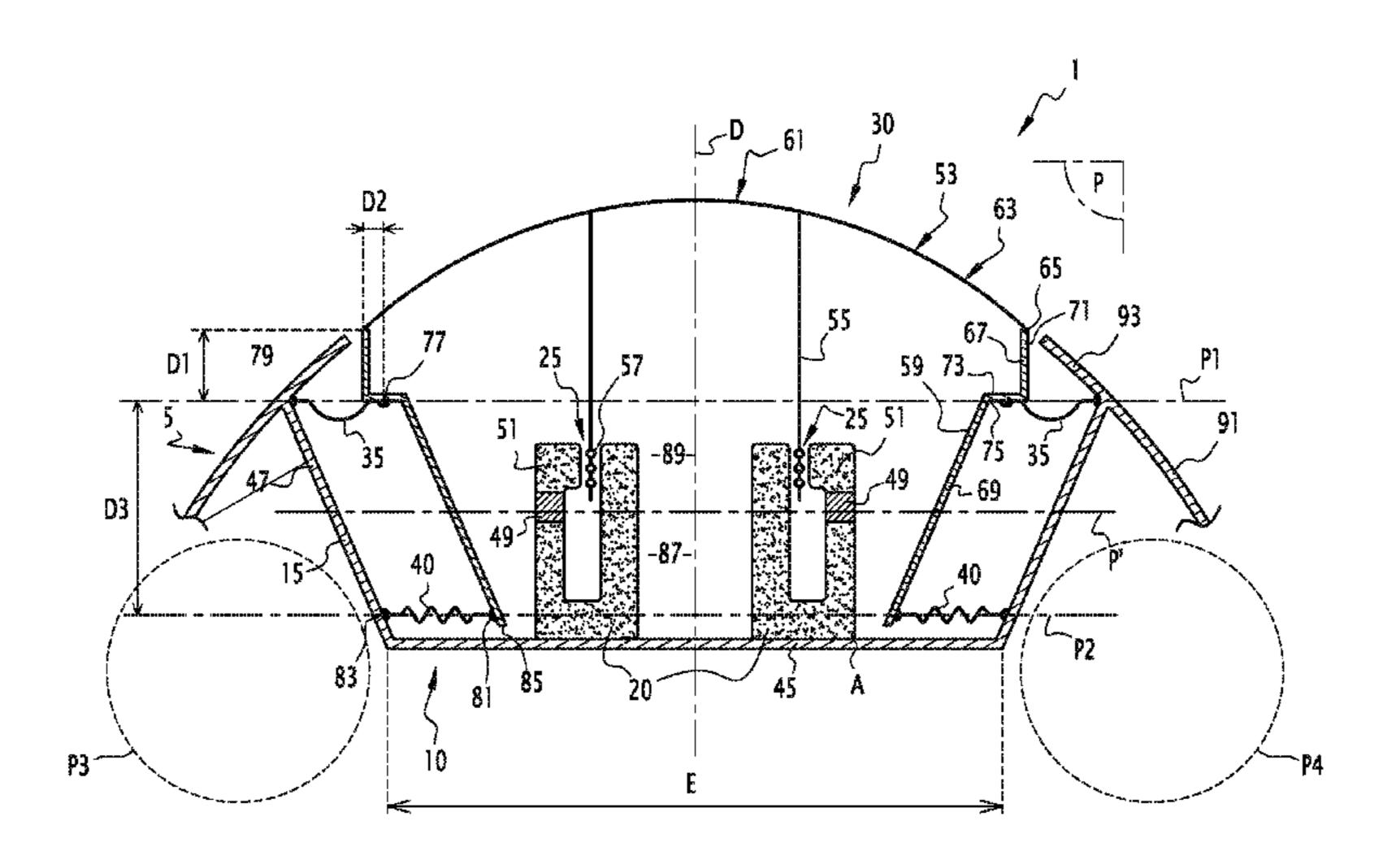
The assembly further comprises at least one connecting member (59) secured to the diaphragm, the second joint including a radially inner attachment point (81) attached on the connecting member, and a radially outer attachment point (83) attached on the chassis.
