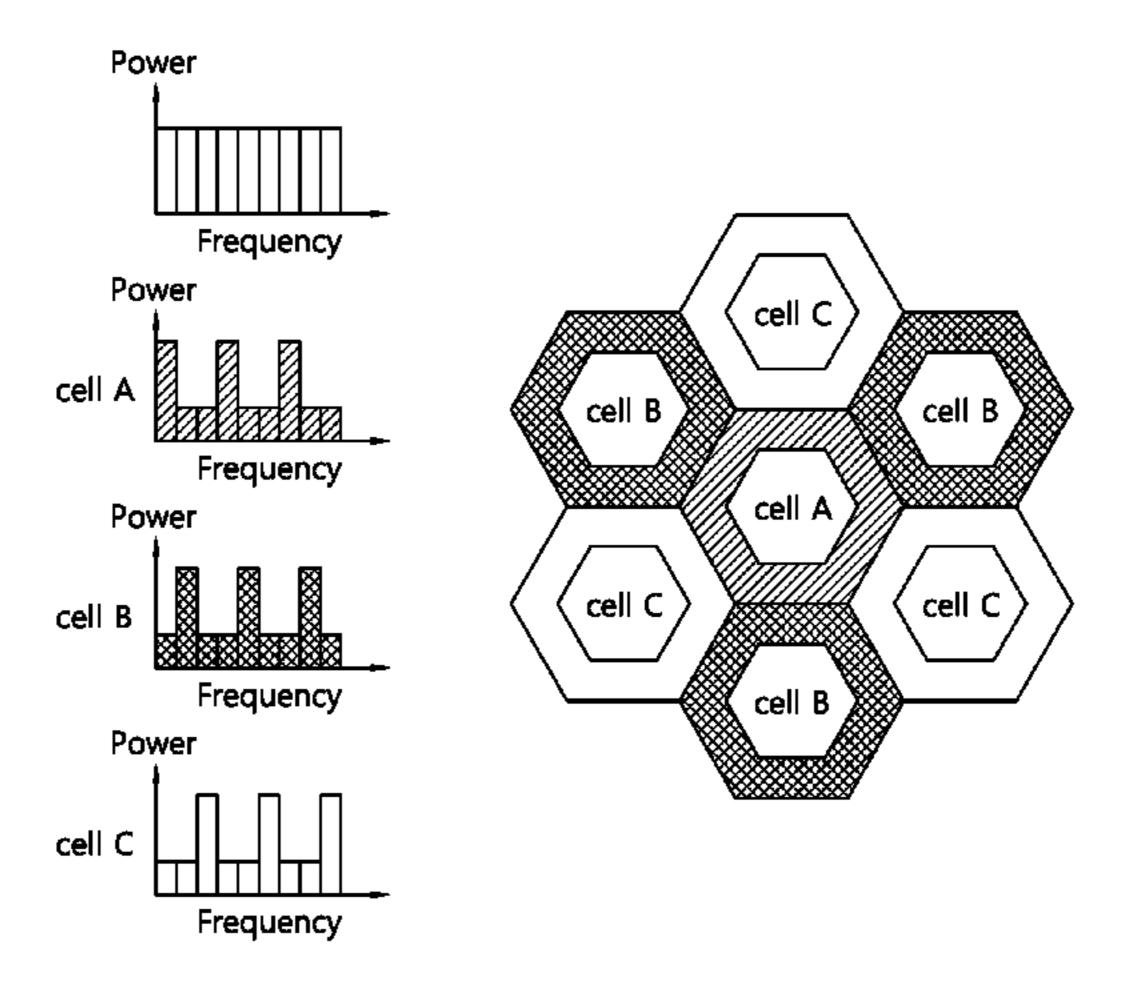
of the signal, and the probability information; and transmitting the interference signal information to an adjacent cell.
