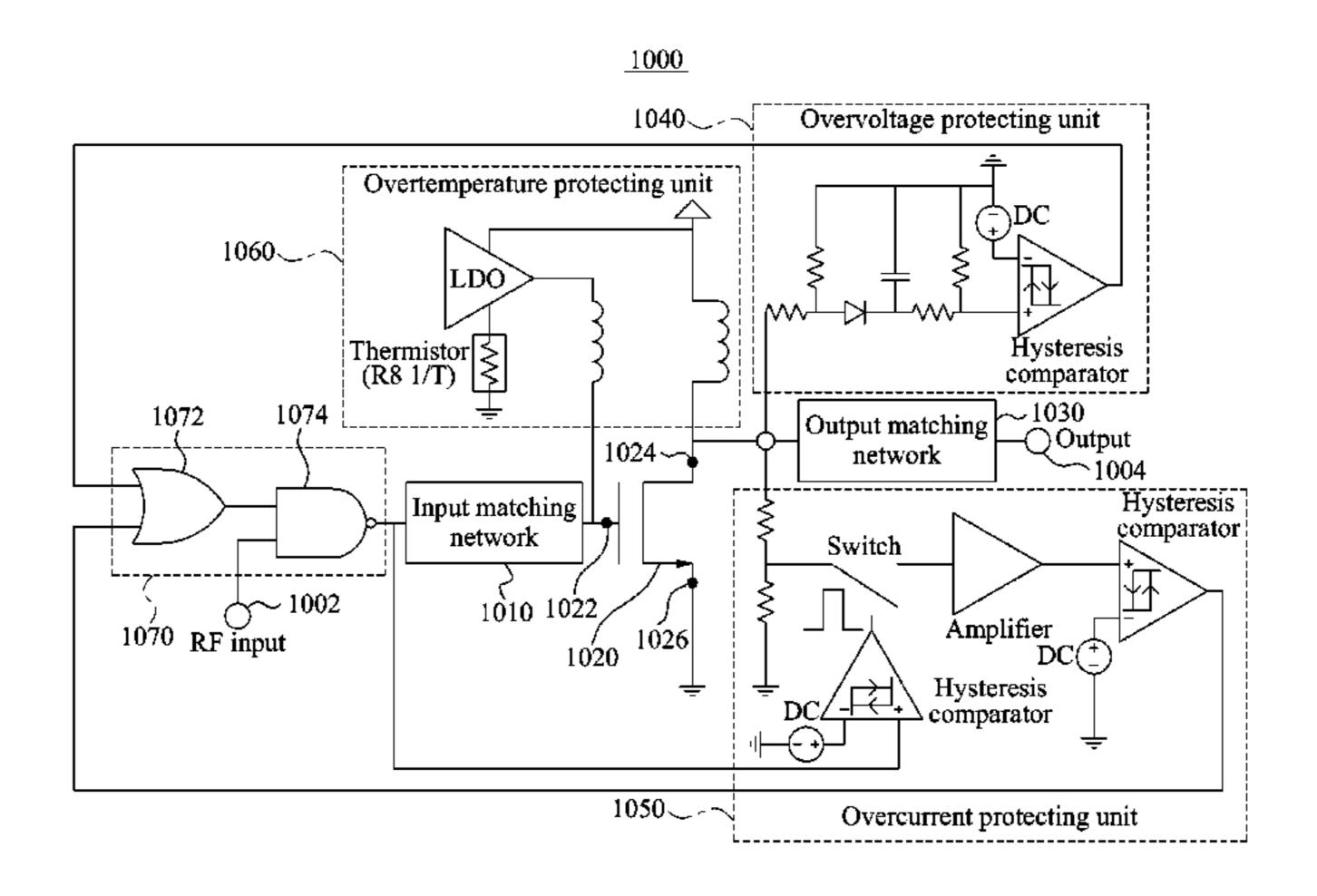
an overtemperature using a thermistor having a resistance that changes as a temperature of the thermistor changes.
