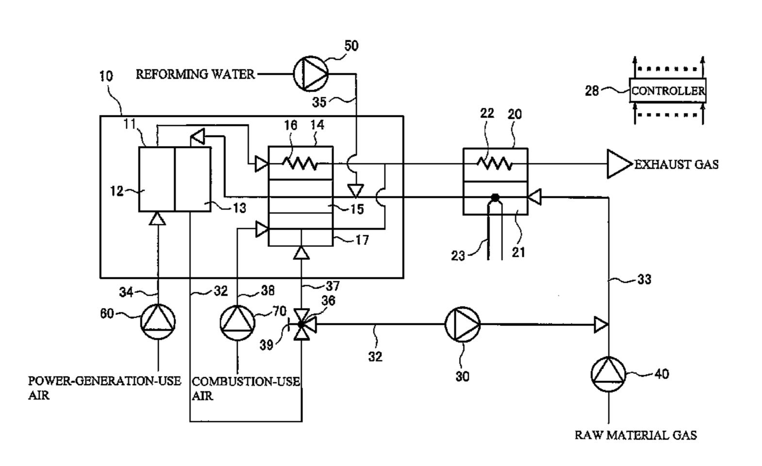
as a heat source, the exhaust gas containing at least combustion heat from the combustor.
