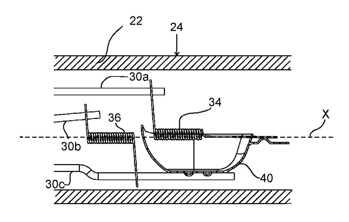
flux of 800-1,000 lm is emitted from the lamp 10. Both the first and the second filament wire 34, 36 are comprised of a filament wire wound in a winding structure around a filament axis, where the number of winding turns for each of first and second filaments 34, 36 is 16-23.
