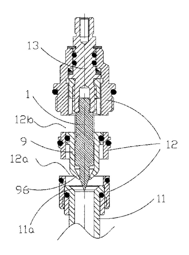
form a cold water inflow space with an inner chamber of the spray nozzle, and form a cold water jetting outlet with the cold water outlet of the spray nozzle, wherein the position of the spray needle in the axial direction of the jet valve core is fixed, and the position of the spray nozzle in the axial direction of the jet valve core is adjustable.
