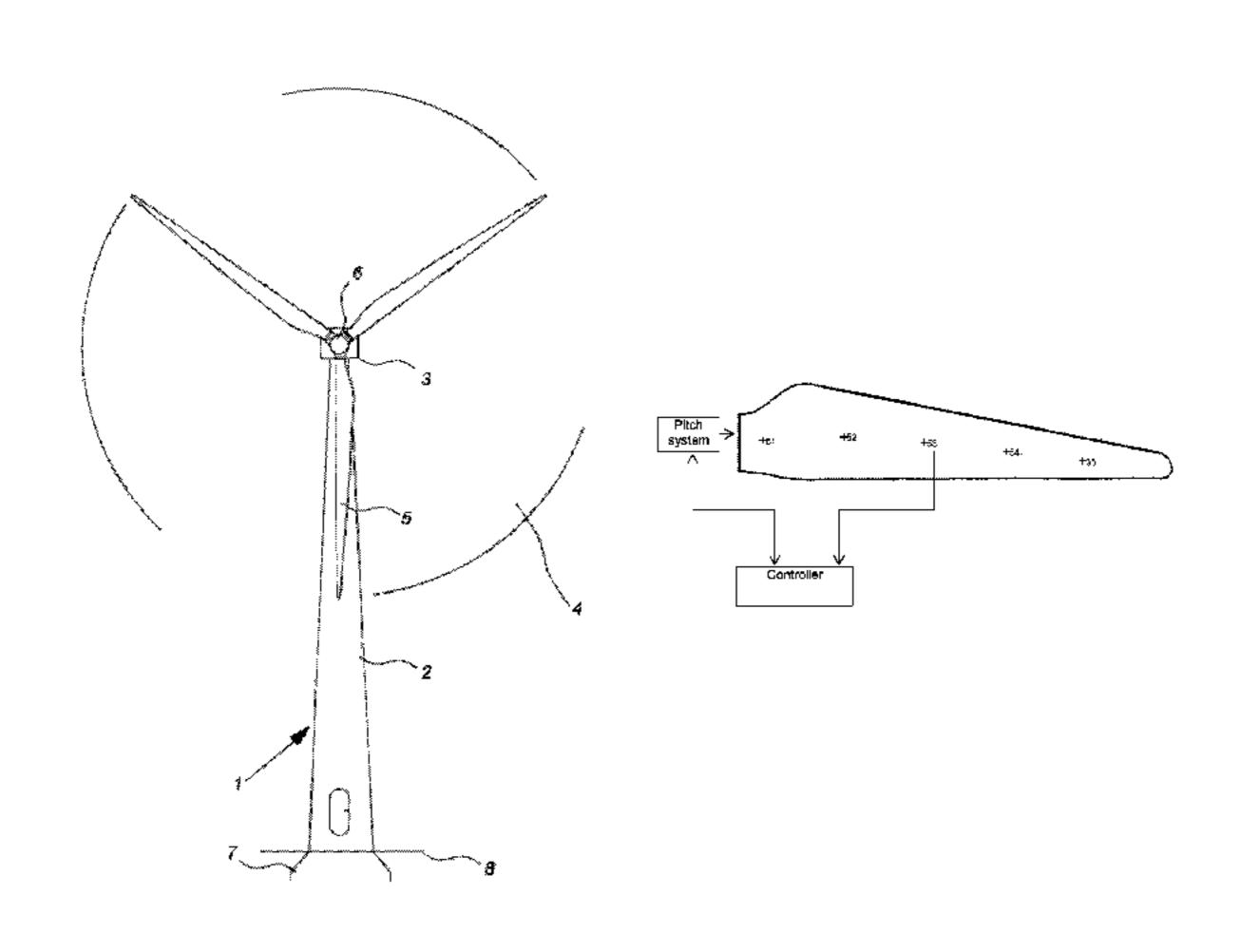
the blade to be excited based on the location of the foreign material by the controller; and excite the blade to the resonance mode; wherein the resonance mode is one higher than the first order resonance mode. The present invention also relates to a wind turbine using the method.
