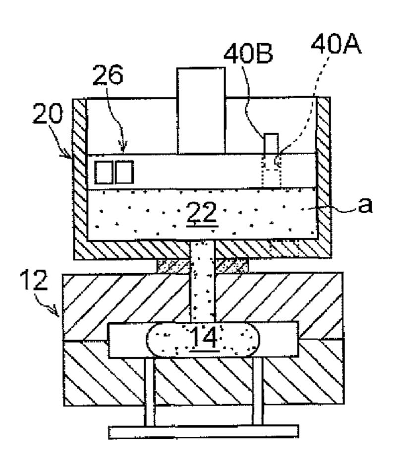
toward the pattern forming space side of the mold by moving the piston toward the foamed kneaded material side.
