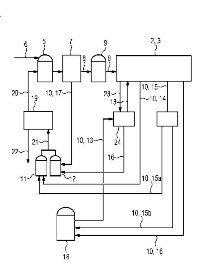
quantity having a first degree of contamination and at least a second partial wastewater quantity having a second degree of contamination are formed in the process. The second degree of contamination is higher than the first degree of contamination. The first partial wastewater quantity and the second partial wastewater quantity are mixed together in such a manner that a combined process wastewater is produced, which is fed to a wastewater treatment plant.
