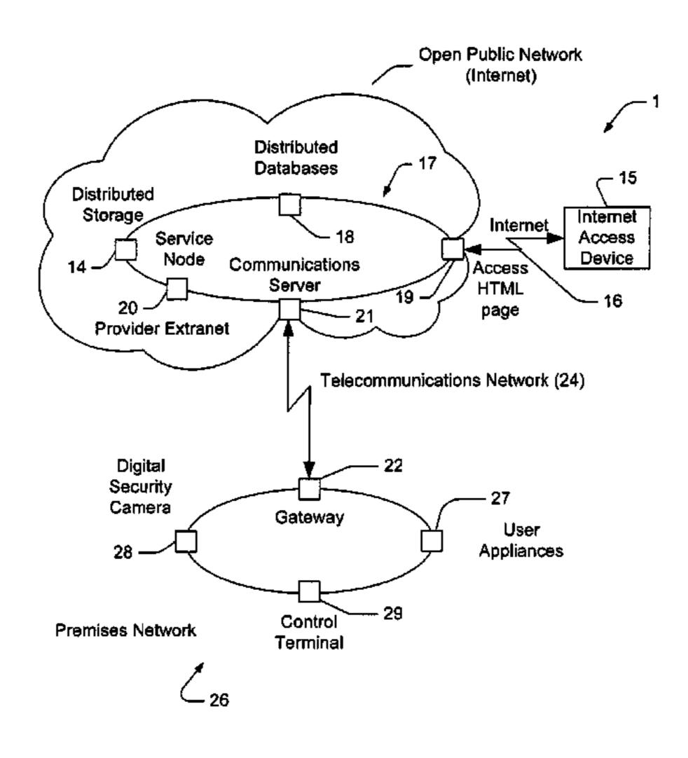
predetermined one of the connection gateways to control and/or monitor the operation of the security device. The extranet can ideally be implemented as a Virtual Private Network (VPN) across an Internet substrate.
