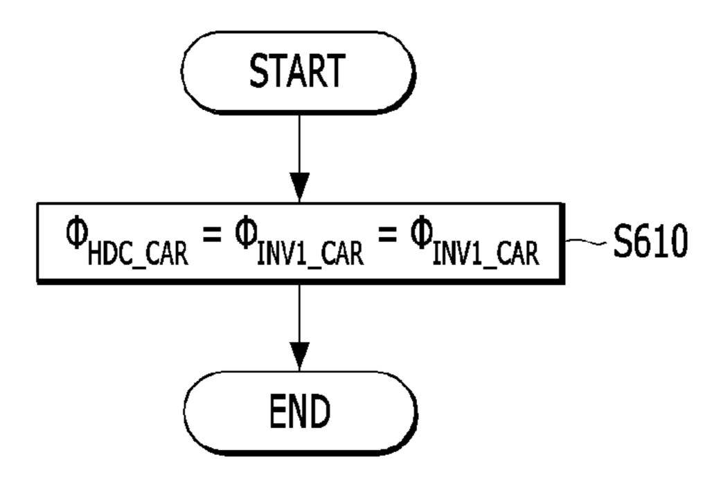
$\begin{array}{l} \Phi_{HDC\_CAR} : \text{ PHASE OF PWM CARRIER FOR HDC SWITCHING} \\ \Phi_{INV1\_CAR} : \text{ PHASE OF PWM CARRIER FOR INV1 SWITCHING} \\ \Phi_{IVN2\_CAR} : \text{ PHASE OF PWM CARRIER FOR INV2 SWITCHING} \\ \end{array}$
