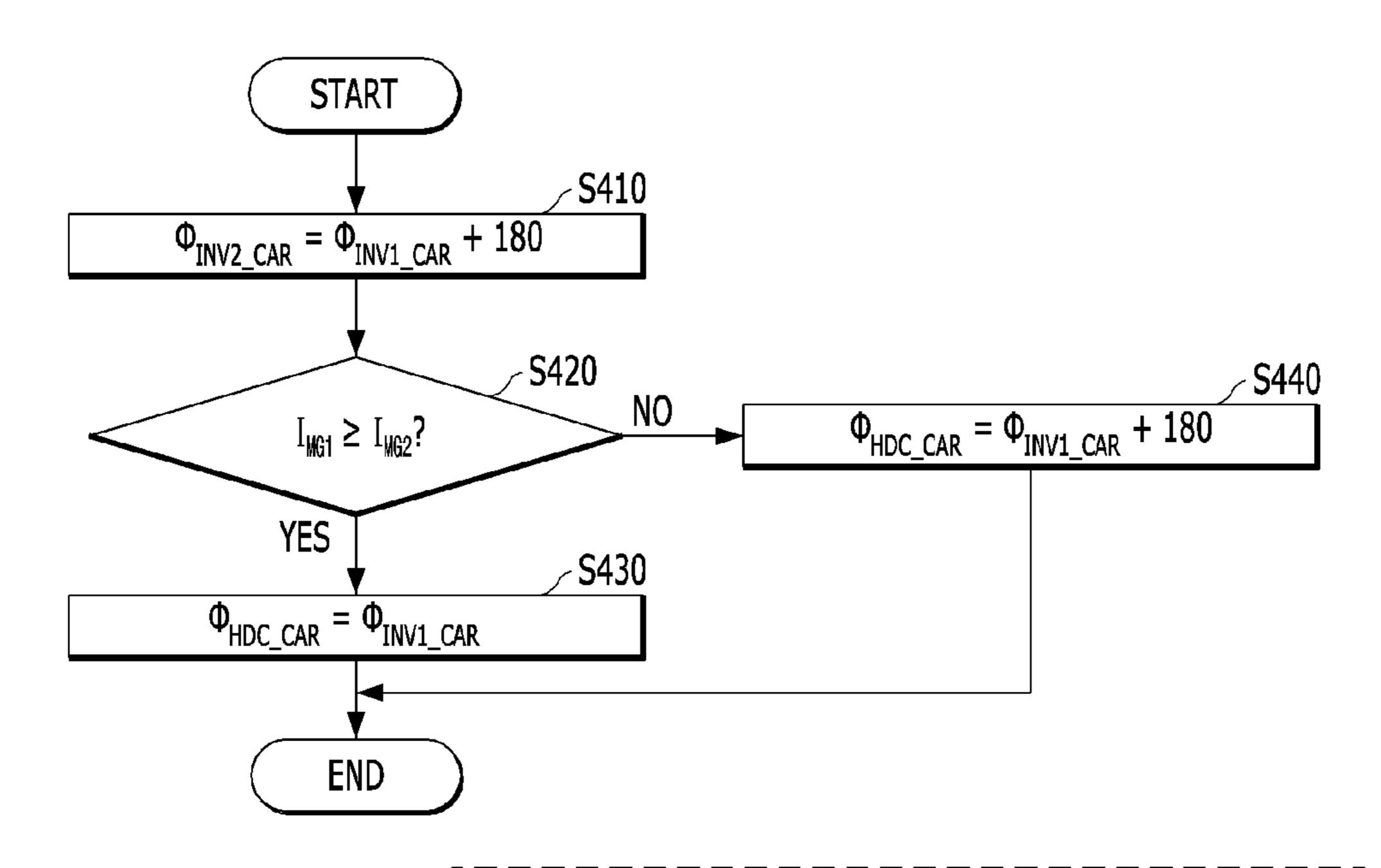
Φ<sub>HDC\_CAR</sub> : PHASE OF PWM CARRIER FOR HDC SWITCHING Φ<sub>INV1\_CAR</sub> : PHASE OF PWM CARRIER FOR INV1 SWITCHING Φ<sub>IVN2\_CAR</sub> : PHASE OF PWM CARRIER FOR INV2 SWITCHING
