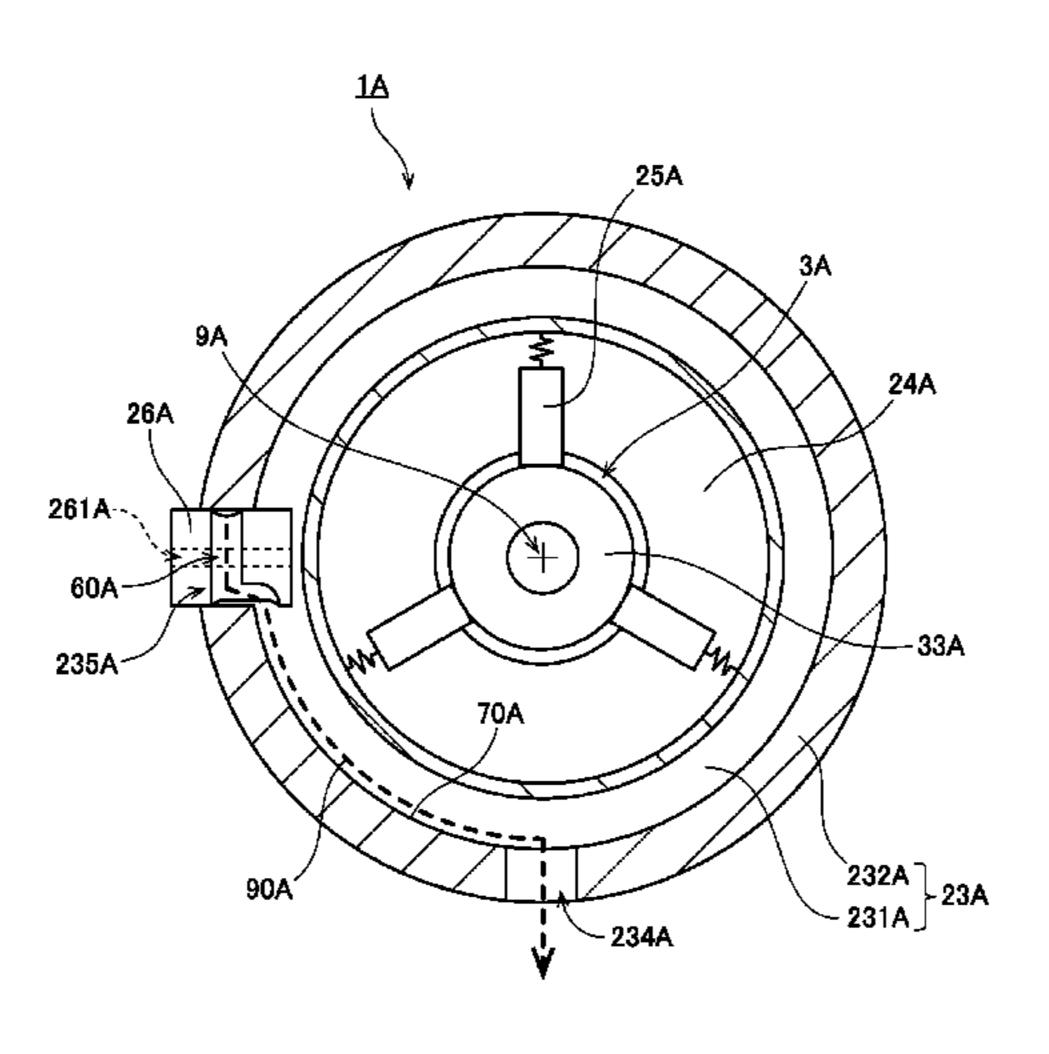
cover. The flow path surface continues from a portion that opposes the flow path groove on a lower side of the flow path groove to the through-hole.
