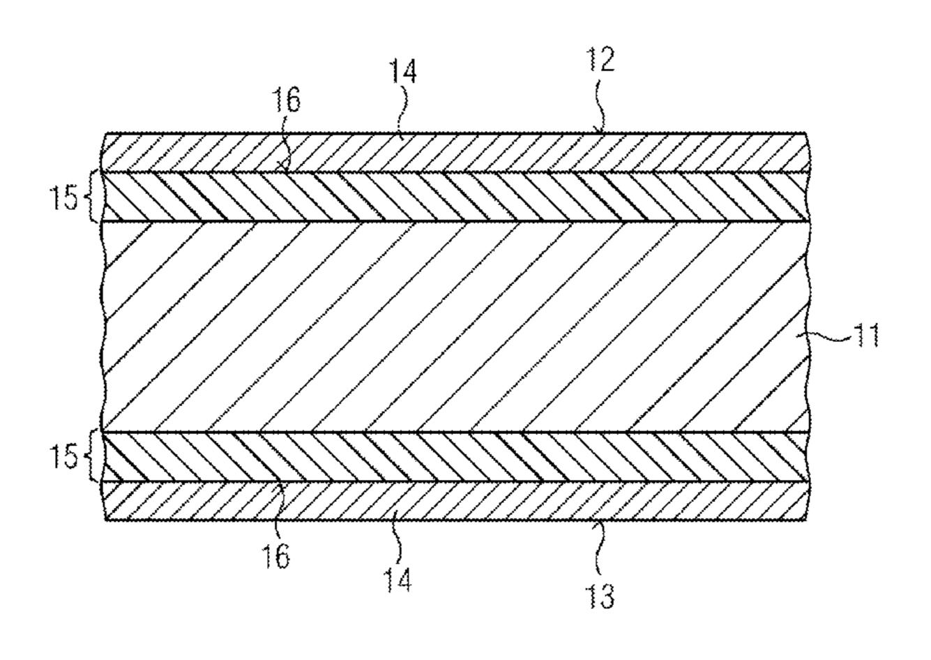
the at the at least one surface is converted into an associated metal oxide to form the layer including the metal oxide, and a residual content of the metal of the metal oxide remains in the diffusion zone.
