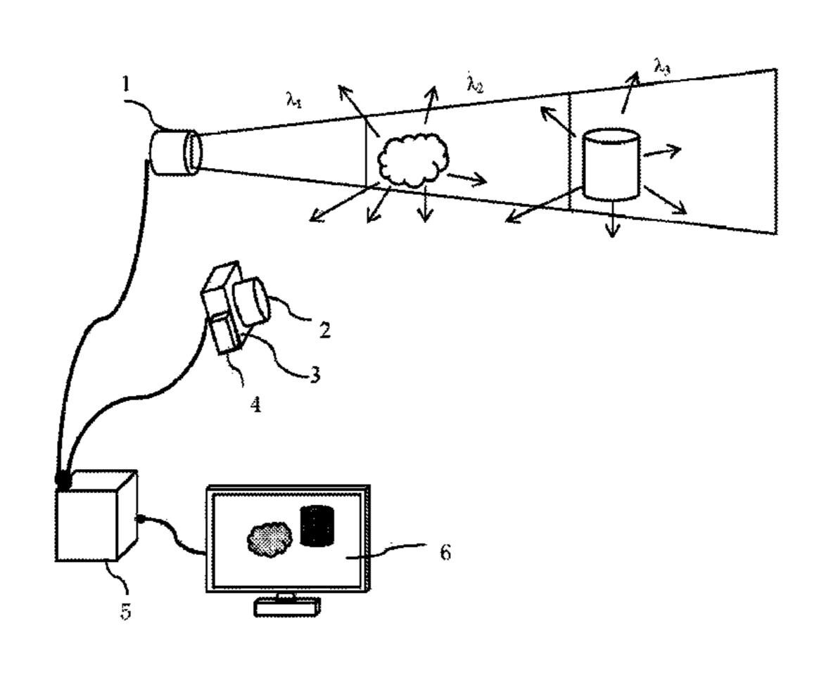
sensor through the optical band-pass filter, to form an image on the image sensor. The image sensor performs exposure imaging three times in succession for the reflected light of the same pulse under the action of the electronic shutter. The data processor analyzes the three images to obtain contour information and distance information about the object. Finally, the display terminal displays results.
