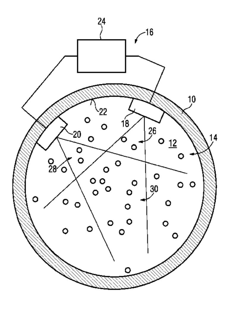
measurement signal characterizing the concentration of the coal particles is provided, wherein an autocorrelation function of the measurement signal is determined and at least one distance value characterizing a distance of a point of the gas flow belonging to the concentration from the microwave sensor is determined in dependence on the autocorrelation function.
