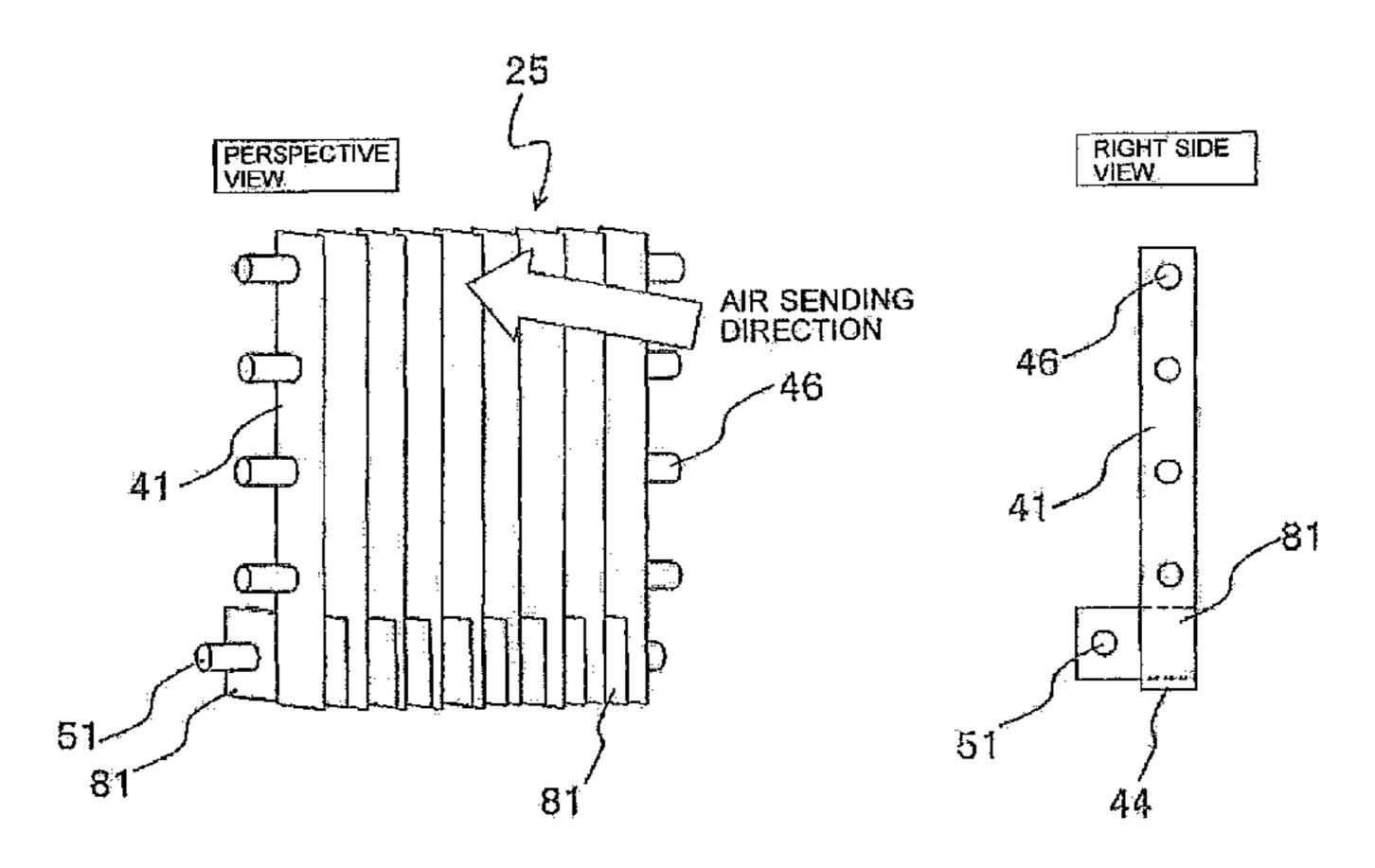
the heat transfer fins and on a leeward side of the heat transfer fins.
