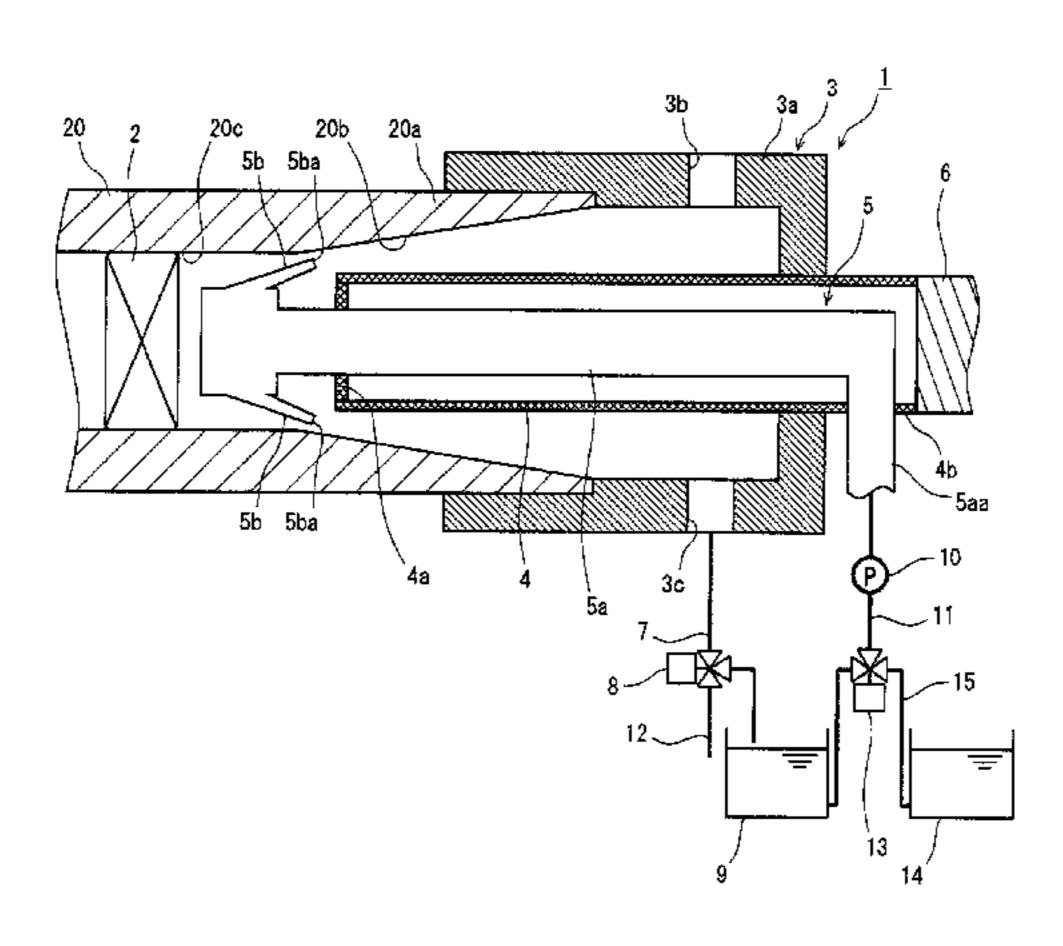
facilitates discharge of the solution inside the capsule. The anode is disposed in the inside of the pipe end portion. The supply tube projects from an end of the anode. The nozzles eject a plating solution between the outer surface of the anode and the inner surface of the pipe end portion.
