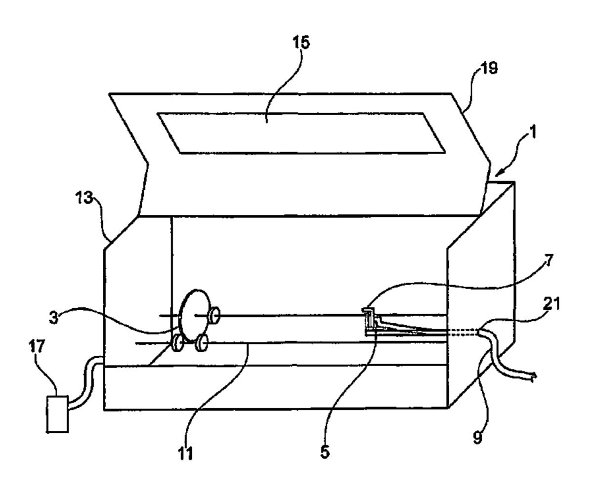
form of an aerosol in the direction of the sample receiving installation, wherein the device has an installation for controlling a reproducible pressure of the propellant medium during the spraying of the test organisms and also the use of a device according to the invention.
