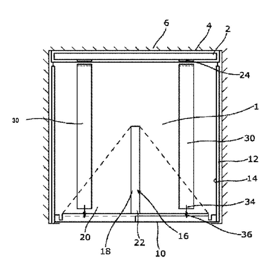
bottom bar, via a spring (36). This connects to keep the strip(s) in tension, to enable ease of rolling of the curtain.
