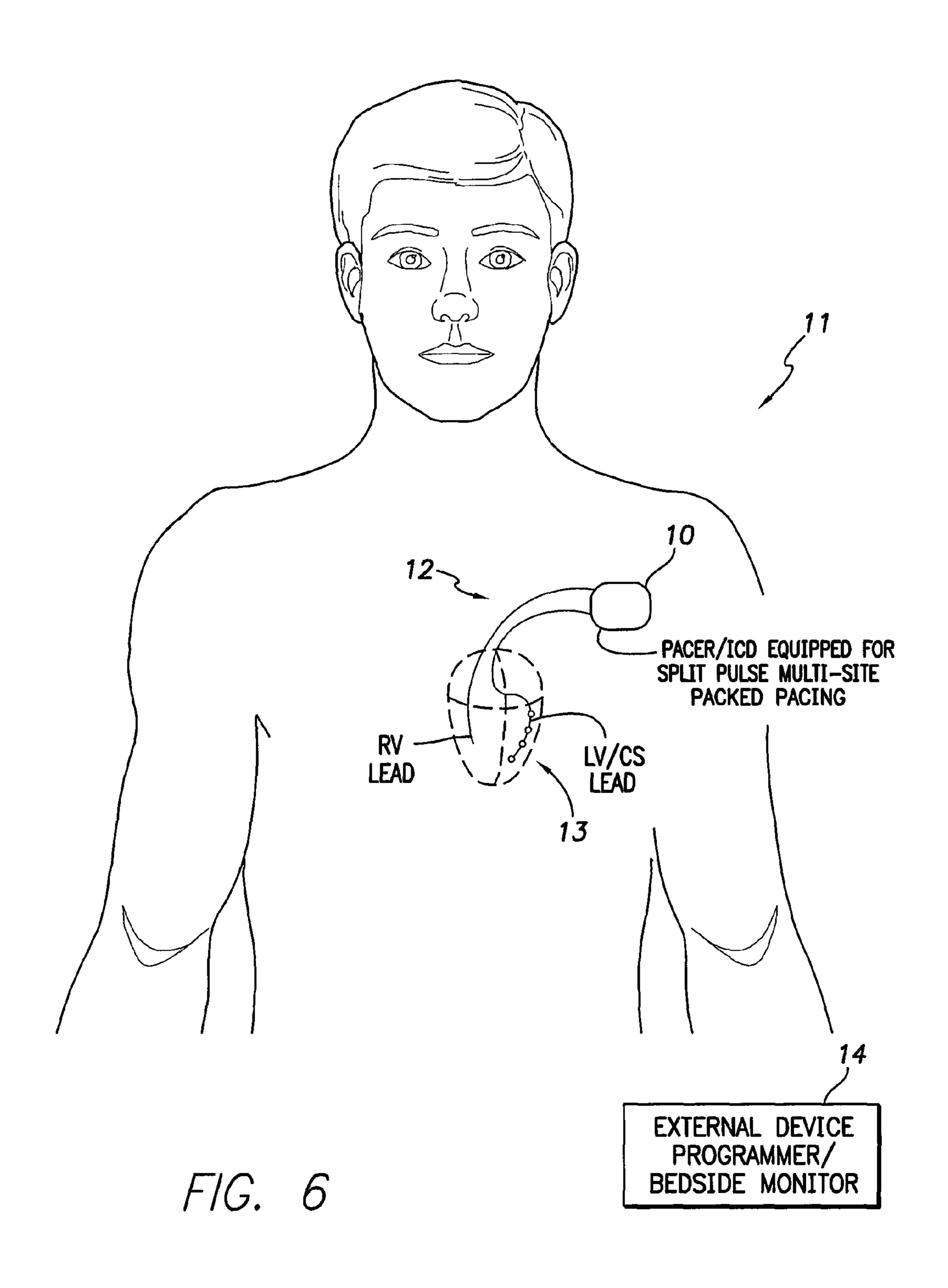
OVERVIEW OF "NEAR SIMULTANEOUS" PULSE PACKING USING SPLIT OR BIFURCATED PACING PULSES
