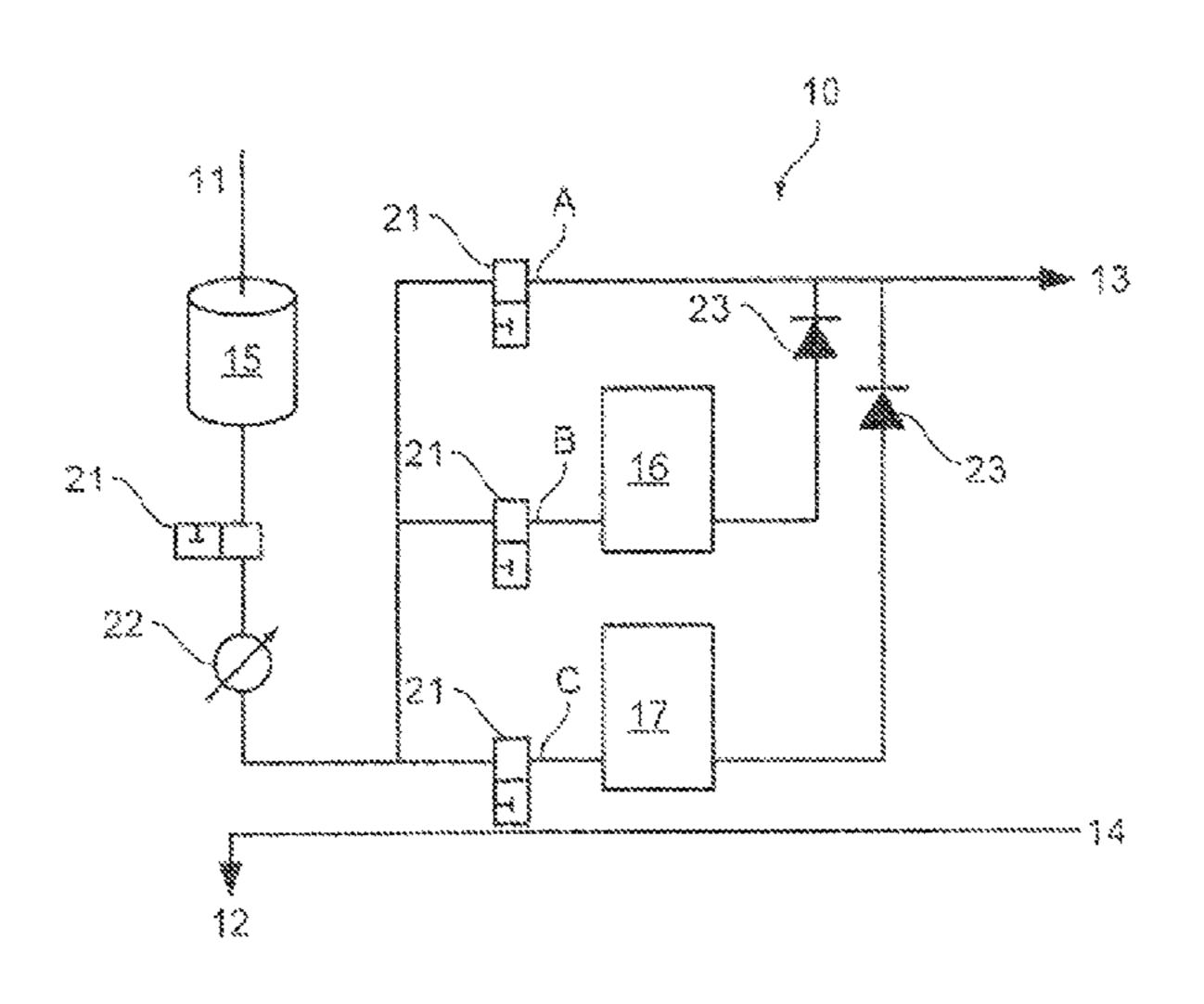
temperature control, a disinfectant is selectively added to the temperature control liquid supply upstream of the temperature control device.
