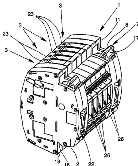
through an opening in the terminal housing, and by movably disposing the securing element with the aid of an actuation element into a terminal position in which the terminal bevel acts against an inner edge of the wall opening in the mounted state of the connection terminal.
