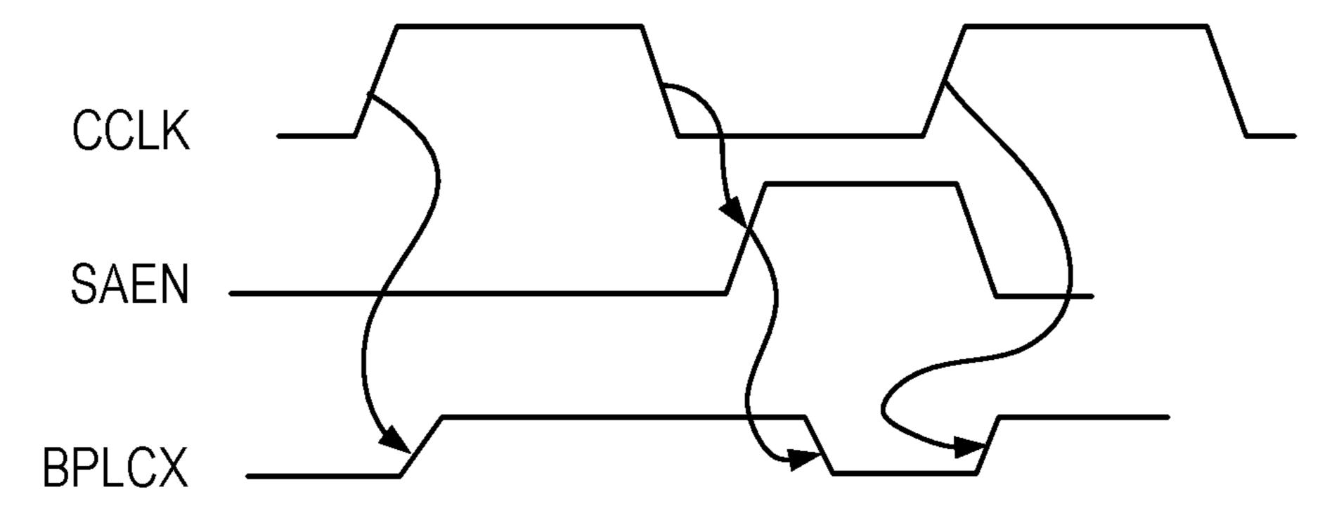
Even when VDD2>>VDD1, pulse width of BLPCX due to faster interlock circuit fuilt as one pseudo-dynamic NAND gate rather than level shifter and NAND gate
