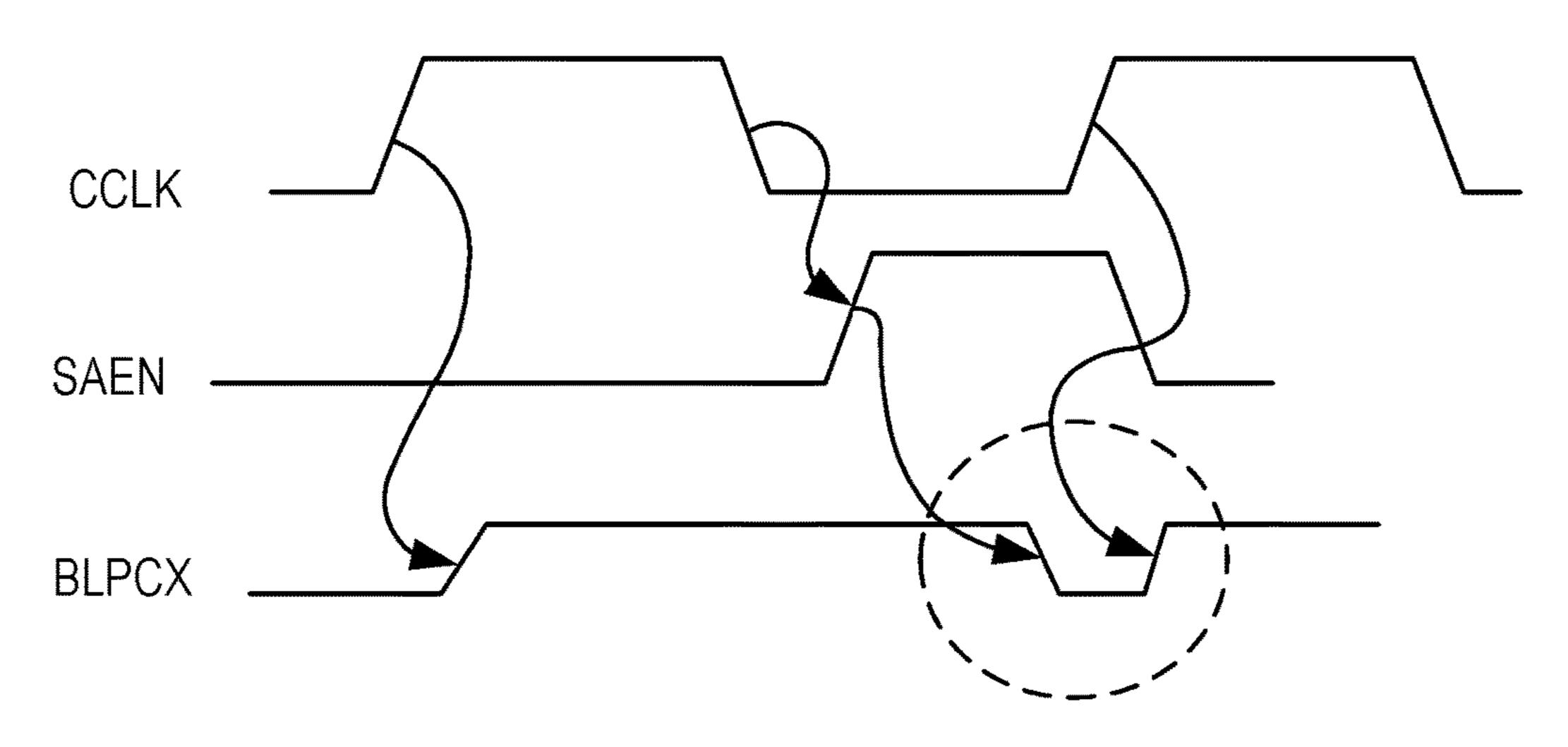
When VDD2>>VDD1, pulse width of BLPCX shrinks until it is not wide enough to precharge the bitlines without slowing down the clocks
