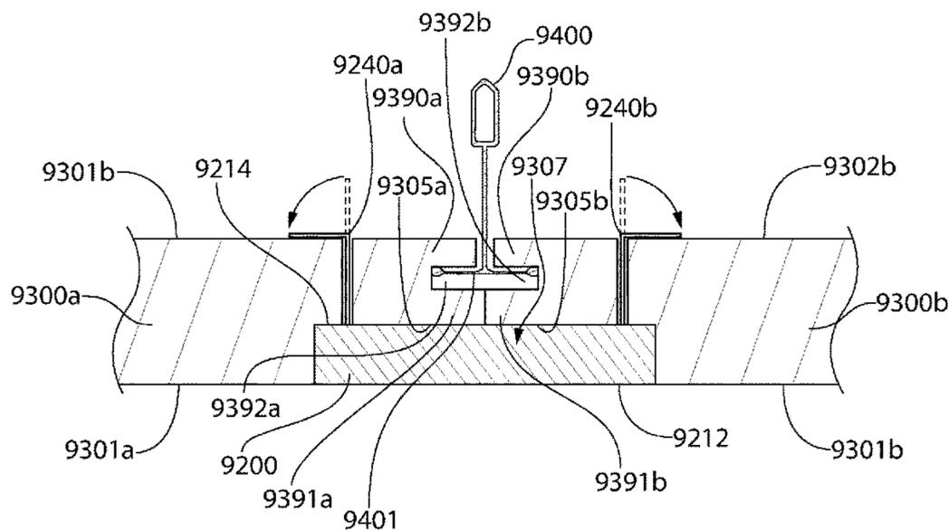
may be of the type that conceals the grid support element on which it is supported. In one alternative embodiment, the light module and a nesting region of the ceiling tile may include corresponding edge profiles to facilitate mating therebetween to enable coupling of the light source to the ceiling tile.
