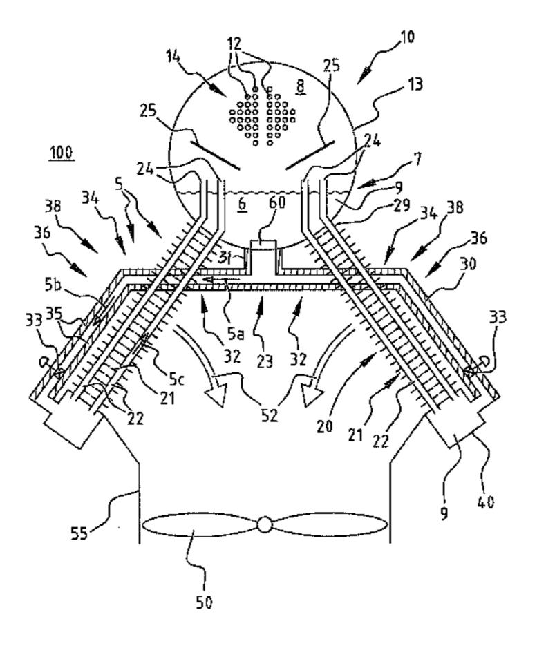
fluidly connects the first heat transfer zone with the second heat transfer zone and has a first transverse portion and a first downward portion that are fluidly connected to each other via a connecting elbow portion. The connecting elbow portion, when viewed in a vertical projection on a horizontal plane, is located external to the box compared to the axis.
