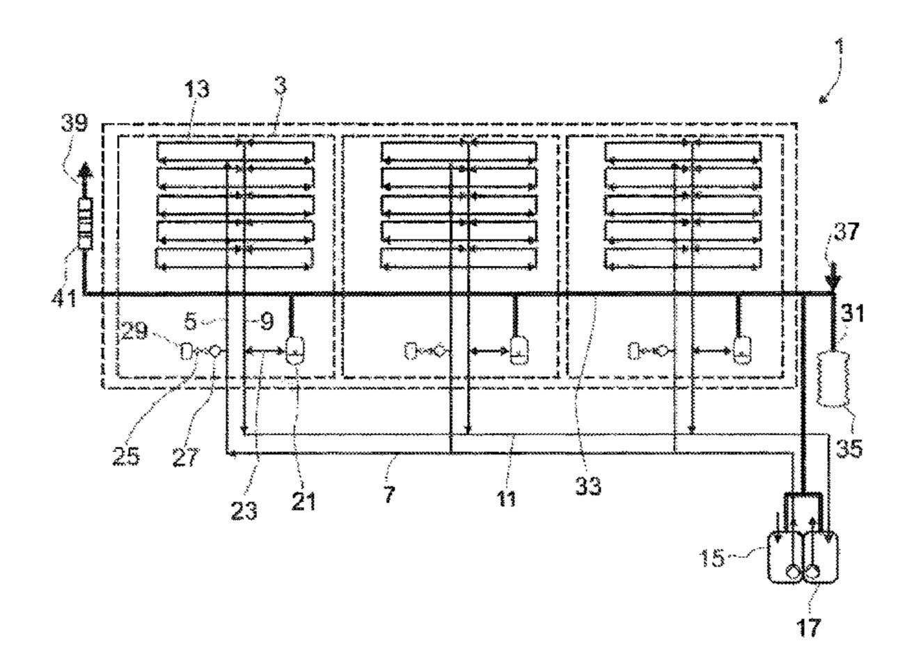
Furthermore, a gas displacement system (31) is comprised, which connects gas spaces in the at least one emptying tank (21) and/or in the store for the heat transfer medium to one another and which has a central gas store (35) and/or a central gas connection (37) and a central exhaust gas outlet (39), through which gas can be discharged into the surroundings.
