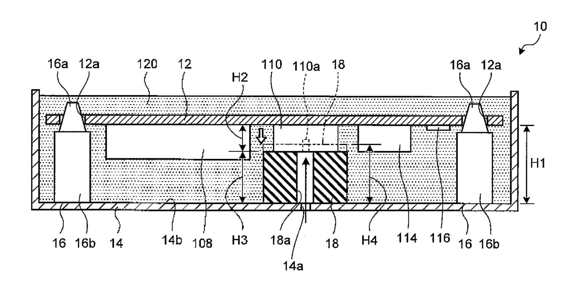
board and by sandwiching the packing between the bottom surface of the case and the sensor.
