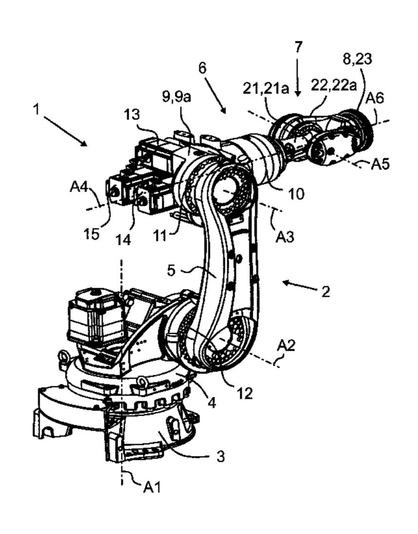
arm extension is offset from and runs parallel to the rotational axis, and a motor shaft of the first hand element drive on the arm extension is perpendicular to and spaced from the rotational axis.
