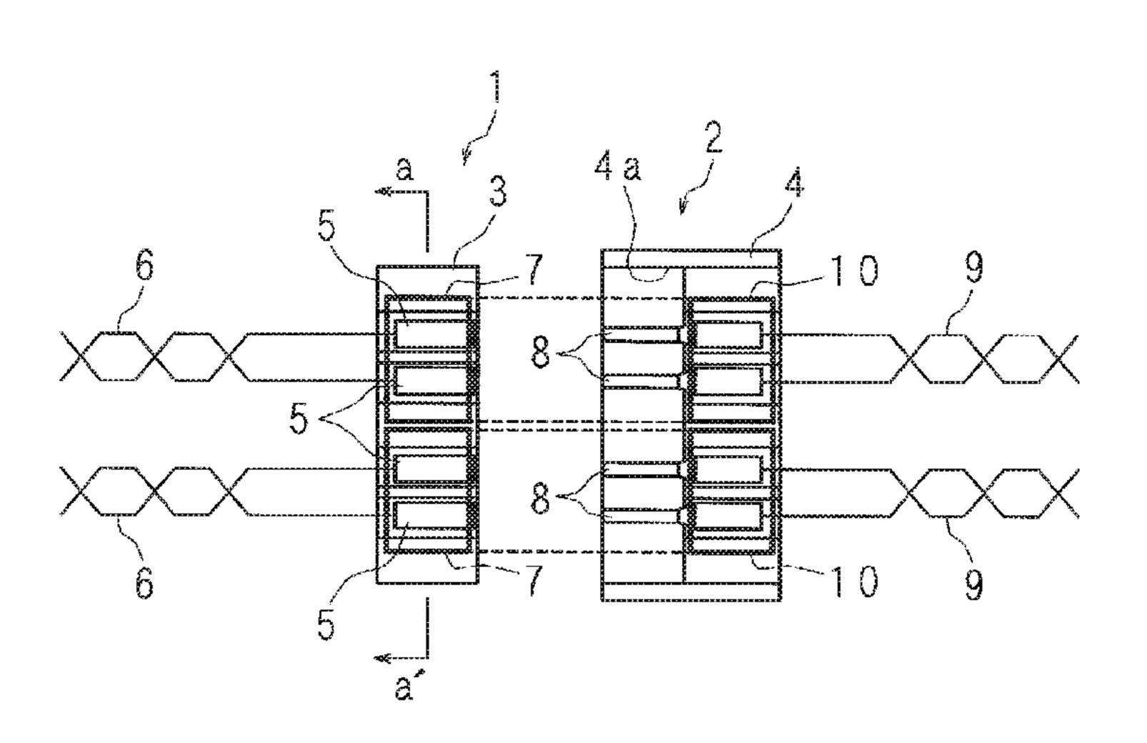
terminal surrounding conductors are respectively connected to the corresponding second terminal surrounding conductors as well.
