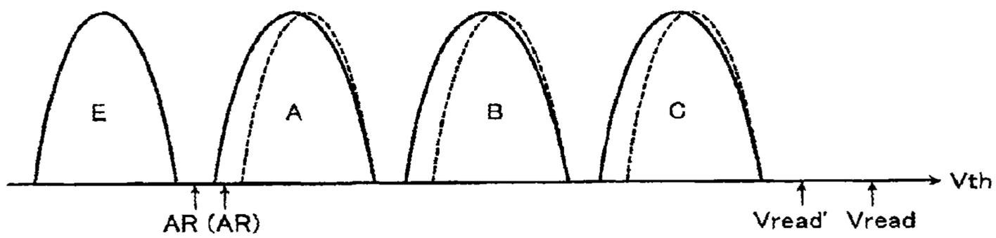
Effect Obtained by Changing Reading Pass Voltage of Adjoining Memory Cells
