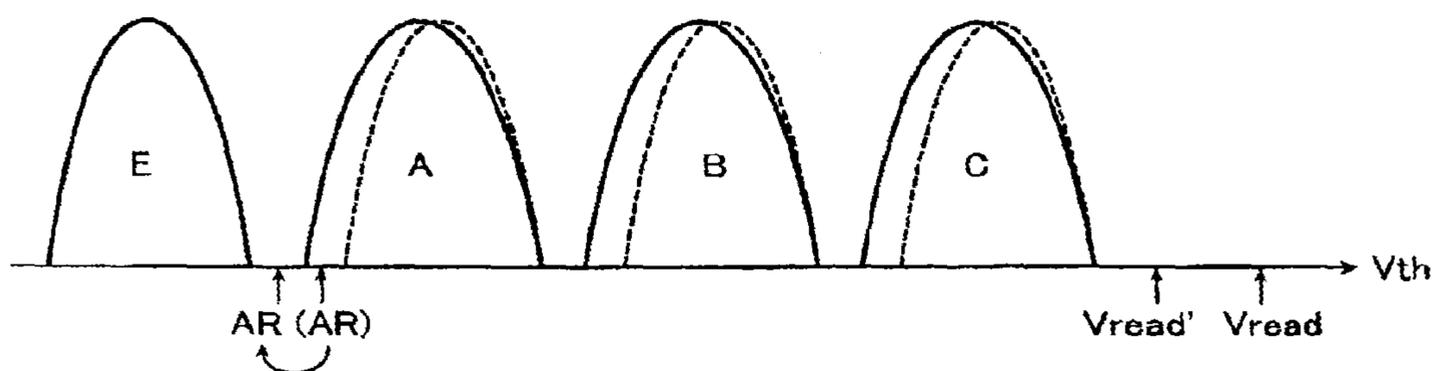
Effect Obtained by Changing Source Line SRC Voltage from 0 V to  $V_{src} +$  Effect Obtained by Changing Reading Pass Voltage of Adjoining Memory Cells
