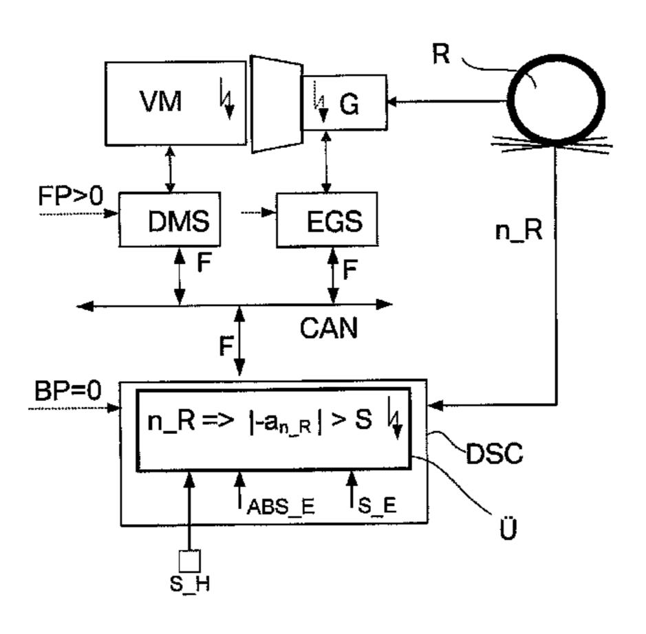
ing module checks for an occurrence of an implausible braking torque, for detecting a defect in the drive system.
