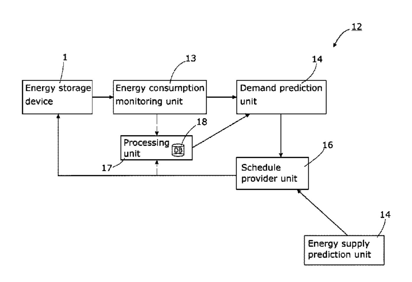
demand prediction that defines a lowermost limit for the supply of energy to the device, and supplying energy to the device in a range defined by the limits specified by the upper energy function and the lower energy function.
