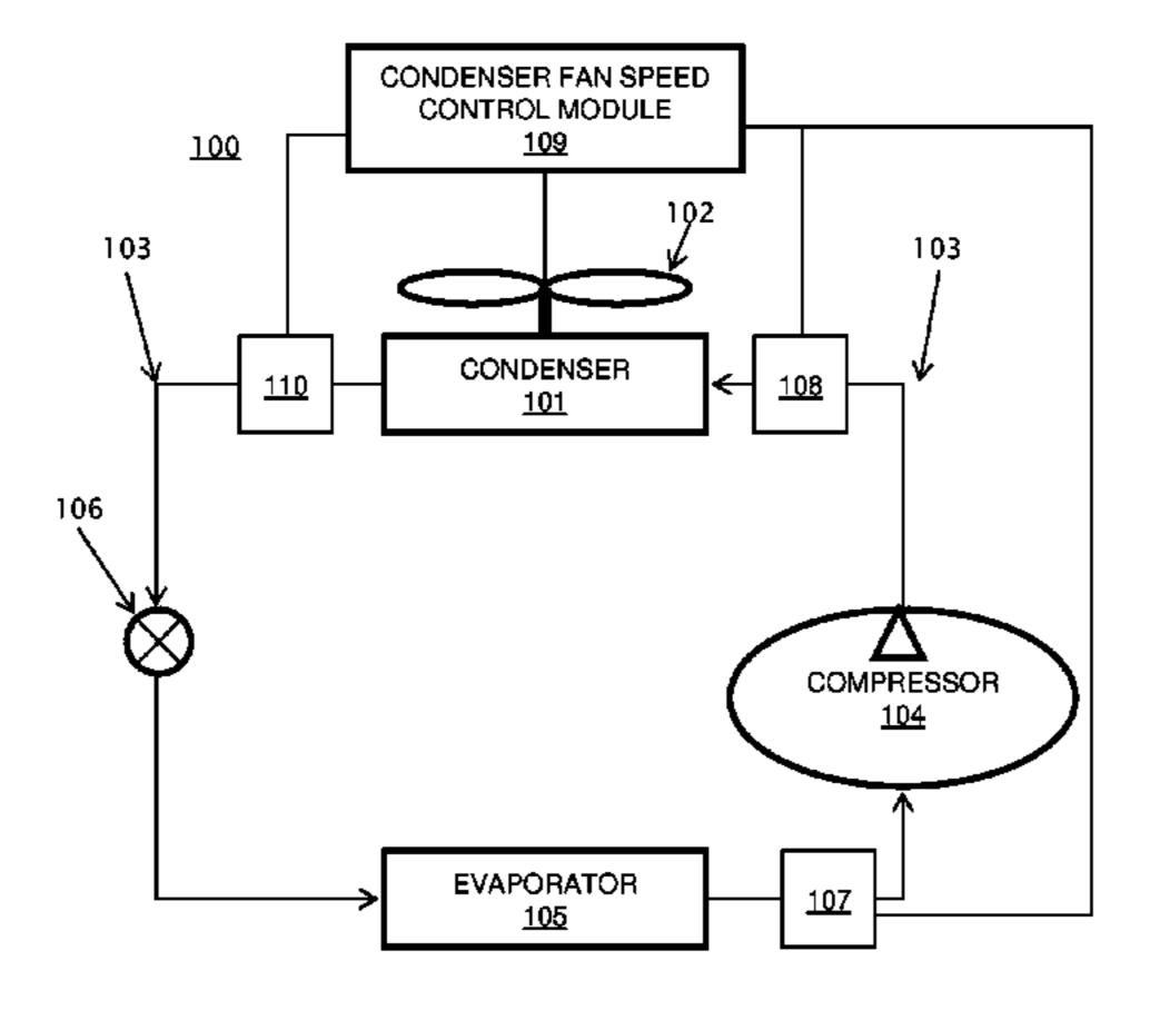
denser fan speed control module; identifying an optimum condenser fan speed based on a vertex of the parabolic curve by the condenser fan speed control module; and controlling the speed of the condenser fan to meet the optimum fan speed by the condenser fan speed control module.
