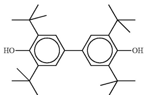
Stabilizers, which can be added, for example, to the liquid-crystalline mixtures in amounts of 0-10% by weight, are shown below.
