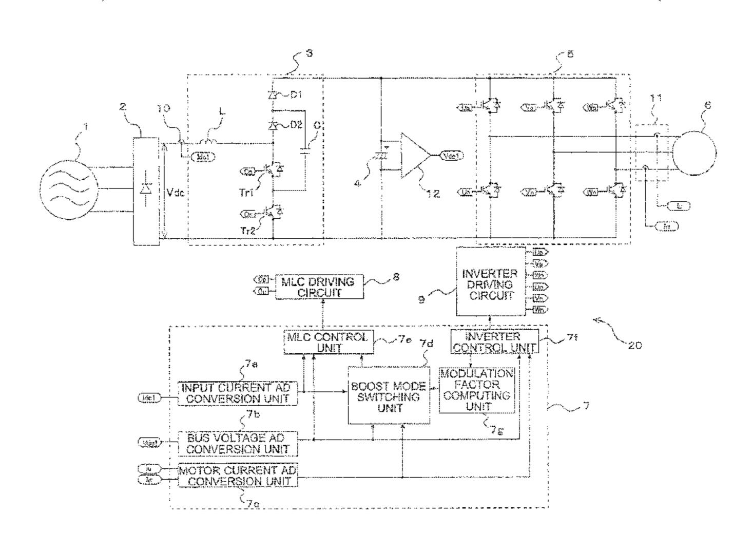
operation status of the motor determined for the purpose of controlling a refrigeration cycle; and an MLC control unit configured to control the MLC circuit based on the switching by the boost mode switching unit.
