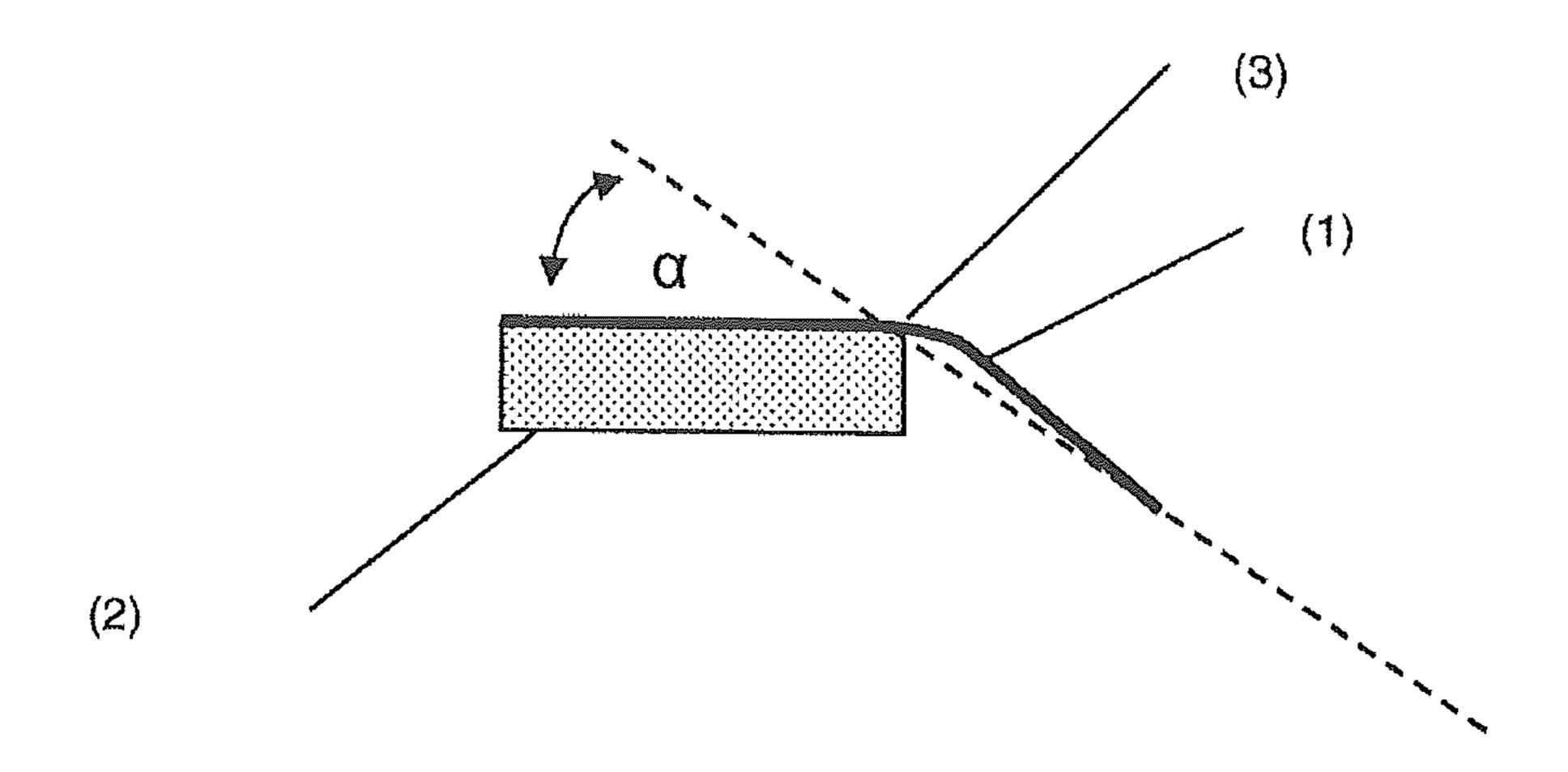
Schematic depiction of the measurement of the flexibility
